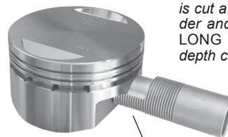
*The threaded portion of the C-Clipper sleeve is cut away to clear the overhanging shoulder and skirt of the piston. Use only with LONG installer, and formed ALUMINUM depth control V-guide, below.*
